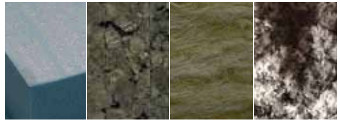
Different types of insulation: XPS, cork, mineral wool, and cellulose
